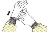
Remove gloves by turning inside-out
